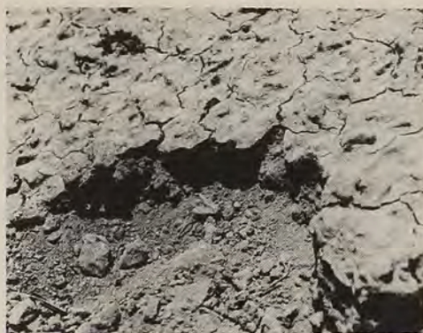
Fig. 2. Bare soil showing a dense crust at the surface, formed when raindrops dispersed the surface soil particles. This resulted in surface sealing and greatly reduced water infiltration.
