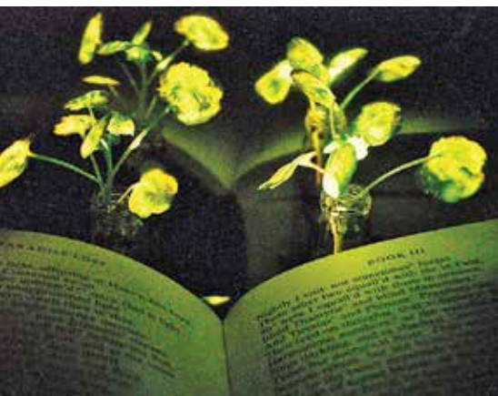
Two watercress plants that have been immersed in light-emitting nanoparticles produce a faint glow in a laboratory at MIT.
