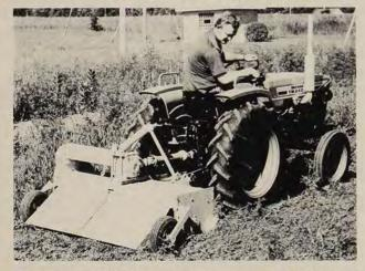
Thousands of Tillits have proven their value in all phases of tiller applications. Tillits are backed by experience in designing and manufacturing agricultural and other mechanical equipment since 1935. Sizes are available in widths from 32" to 84". The model LDT shown above is suitable for use with tractors in the 15-30 PTO horsepower range such as Yanmar, Ford, Kubota, Mitsubishi, Leyland, Suzue and any other of similar specifications. Write for literature.
