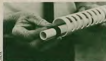
TOP LEFT: Plastic hot callusing pipe consists of two cylinders. The outer cylinder is slotted to localize warm air to graft unions while holding them in place. The inner cylinder separates two heating cables and helps stabilize air temperatures when filled with water. TOP RIGHT: These whip and tongue grafts were callused following 28 days on the hot-callusing device at 80 degrees F. Graft unions are bound with rubber grafting bands.
