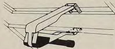
The SELECT model — best for greenhouses because it takes only 2 inches headroom. Clamp-on attachments simplify installation on metal houses.
