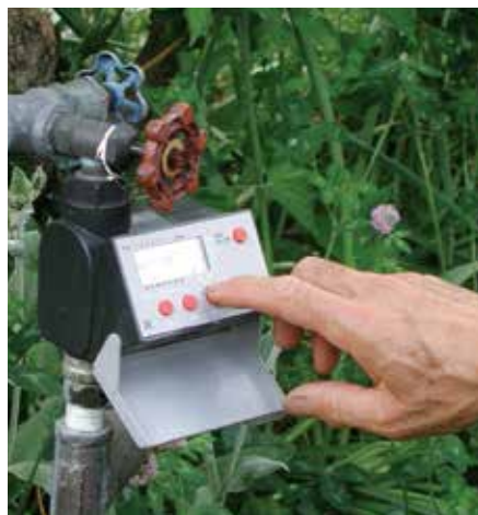
The timer for an irrigation system regulates intervals for watering. Except in warm regions, this unit needs to be brought indoors in winter.
